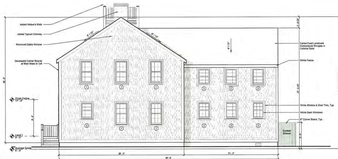
① South Elevation - Mariner Way 1/4" = 1'-0"
