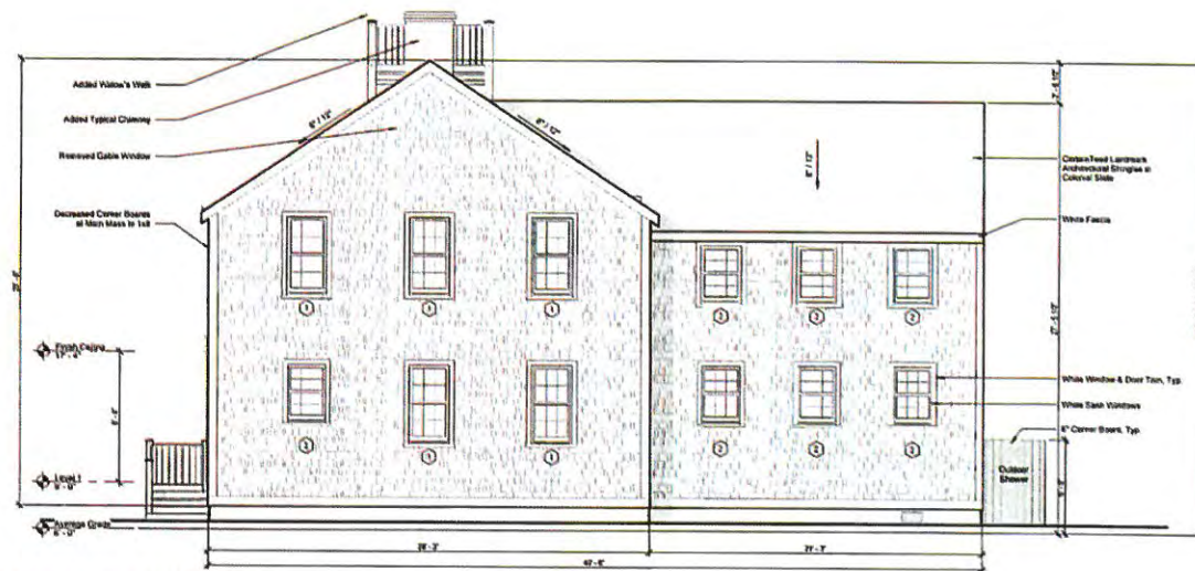
1 South Elevation - Mariner Way 1/4" = 1'-0"
