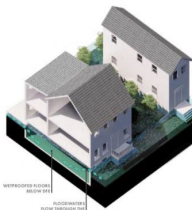
Install Flood Vents
