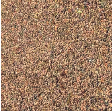
IMPERVIOUS WALKWAYS - TAN CHIPSEAL
