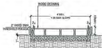
03 BOARDWALK: Section (TYP) Scale: 3/8" = 1'-0"
