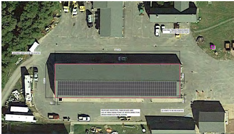
106.2 kW Solar Array: Surfside WWTF
