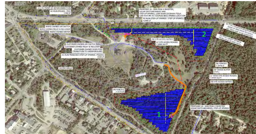
3.8MW Solar Farm (Two Arrays): WWCo "Wyer's Valley"
