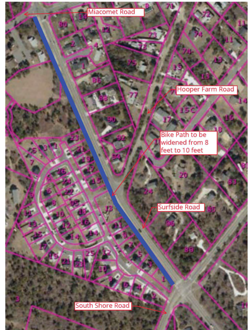
FIGURE 8 - SURFSIDE ROAD BIKE PATH EXPANSION
