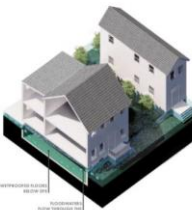
Install Flood Vents
