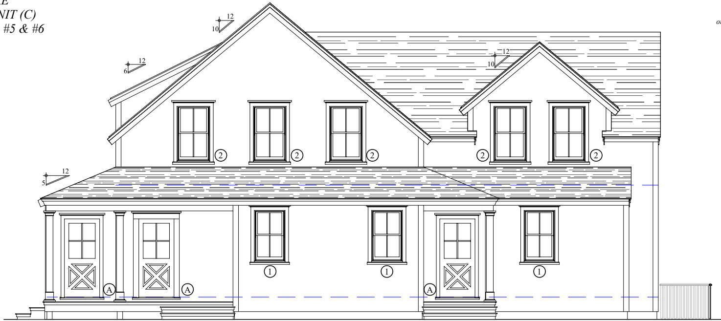
SOUTH ELEVATION - UNIT C facing faregrounds road
